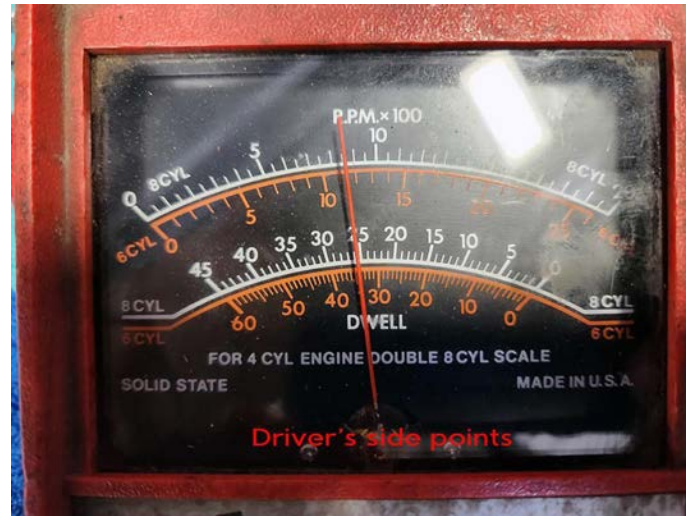
Dwell reading. Note the varying scales. My Lincoln runs as two 6-cylinder engines, so I use the 6CYL scale. Spec is 36° and I have adjusted it to 35°. It will pull itself into spec as the rubbing block wears.
