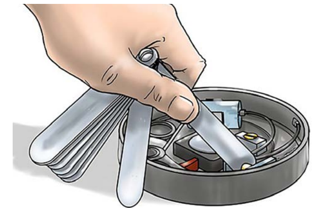
Checking point gap.
