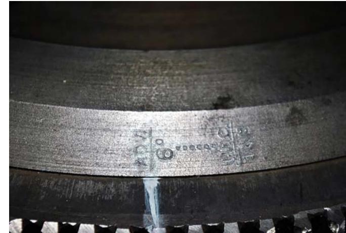
Timing marks on the flywheel can be difficult to see. Highlight them with white paint so they show up with a timing light.
