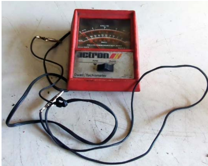
Basic dwell meter is all that's needed. Older units with just two wires are sometimes most effective.
