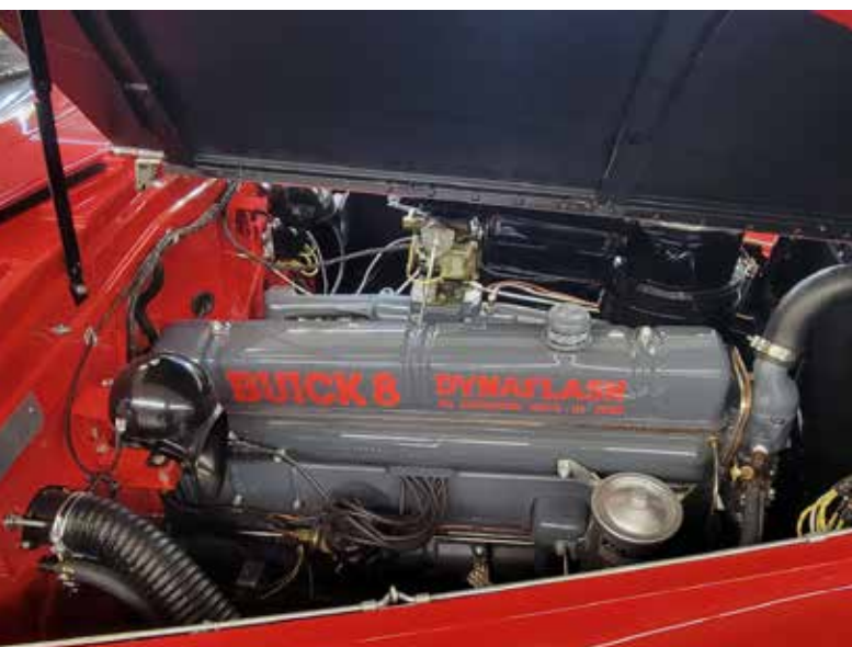
Chief's car uses Buick's biggest and most powerful engine, a 320 cubic inch straight-8
