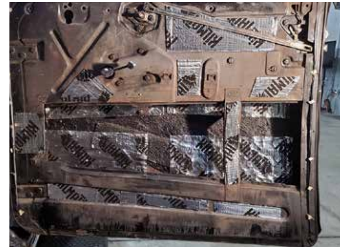
Adding some attenuator mat to the inside of your doors can make a big difference. Note that 100% coverage isn't required.
