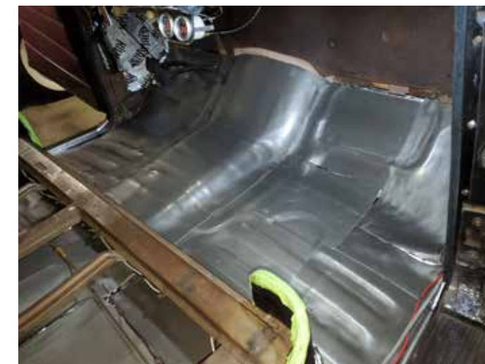
Closed cell foam mats over the attenuator mat.
