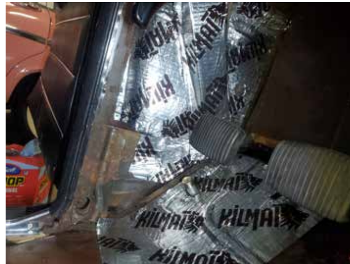
I added some attenuator mat to the kick panels and cowl to help reduce noise in these areas.
