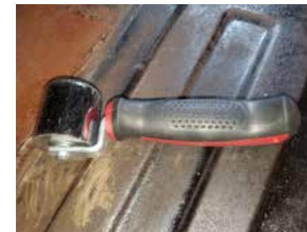
Roller ensures the mats are fully adhered to the floor.
