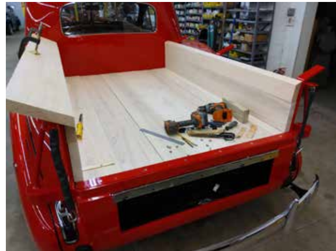
Truck bed being rebuilt with northern ash
