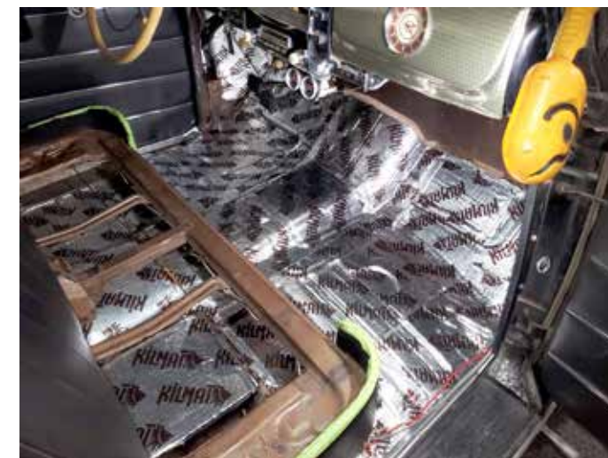
First layer of butyl attenuator mat installed. Note how it hugs the contours of the floor. I probably should have removed the seat.
