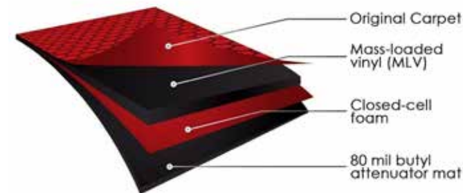
Multiple layers of sound deadening is the most effective way to control noise and heat
