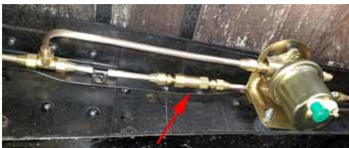
8. Connect the output side of fuel pump to a second T-fitting. You can clearly see how the check valve (arrow) prevents back-flow from the electric pump.
