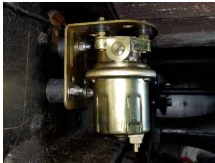
4. Rotary vane pumps are noisy. Using rubber mounting feet can greatly cut down on the noise transmitted into the car (a "Quiet Pack" kit is available, Carter part no. 18-14U, $12.99).
