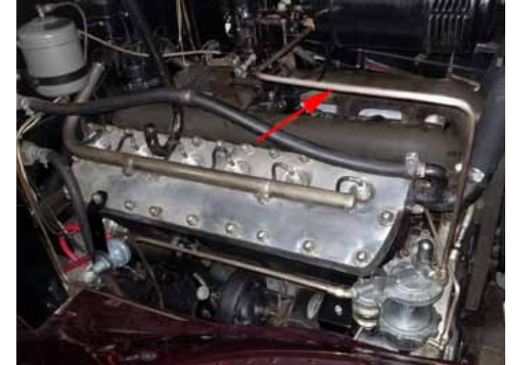
12. Using templates, both the lower and upper (arrow) fuel lines fit perfectly on the first try. Be sure to avoid hot spots! You'll note I also installed spark plug wire conduits, new oil filter lines, and new vacuum lines while I was at it.
