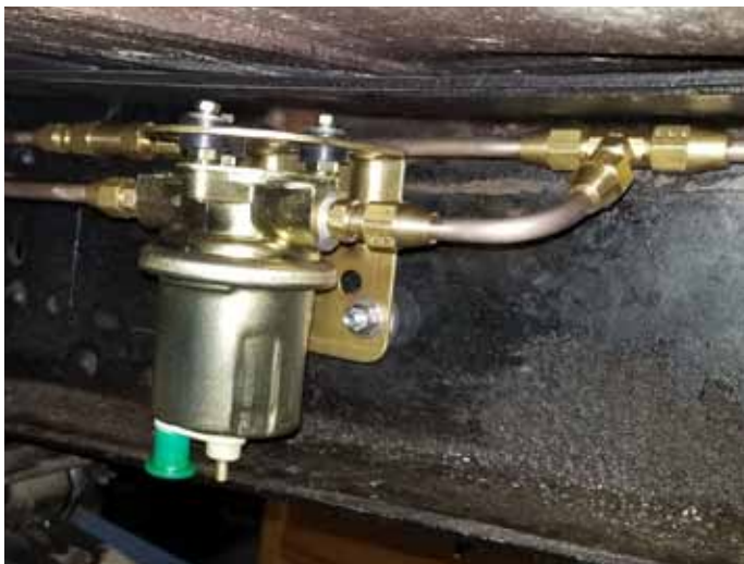
7. Connect the first T fitting to the input side of the fuel pump.
