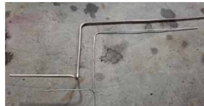
11. Routing the line up to the mechanical pump required some relatively complex bends around the frame. To properly locate those complex bends, I made a template using some wire then duplicated it with tubing. Easy!
