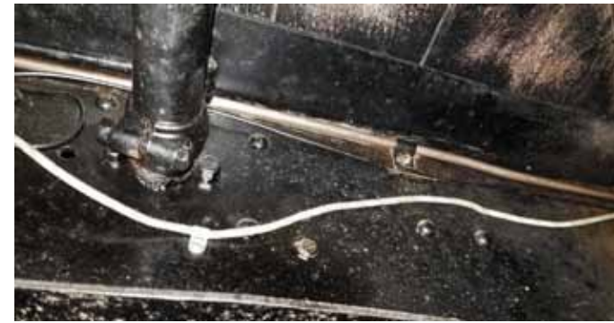
9. Run the line to the mechanical pump up front on the engine. Again, follow the original fuel line's route if possible. I was able to re-use all but one original mounting hole and even reattached the fuel gauge capillary tube in the original clips.
