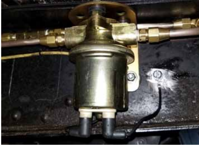
14. Connect power (yellow wire) and ground at the pump.
