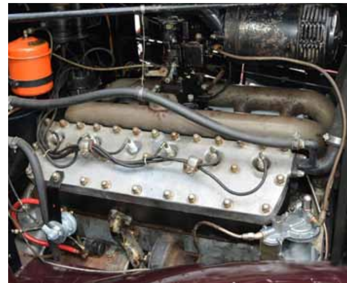
10. This is what I started with—what a mess! The line from the tank was kinked and sat right on top of the water pump. The upper line from the fuel pump to the carburetor was right above the exhaust manifolds and was actually touching the upper radiator hose. Think about the best way to route your lines and get them as far away as possible from heat sources.
