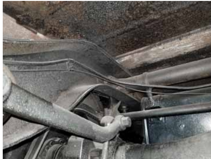
2. Ideal location inside the frame where the fuel lines are located and there's plenty of room. Up here, the pump will be protected from road debris, heat, and moving parts. Note original fuel line and gas gauge capillary tube.
