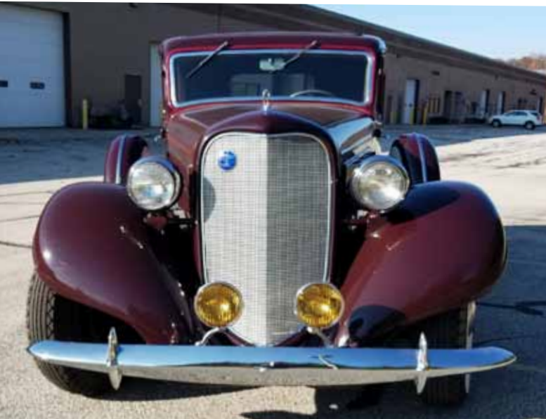
Imposing front-end view with dramatic fenders, mesh grille, and streamlined bumper. Sidemounted spares were optional; fog lights added by owner.
