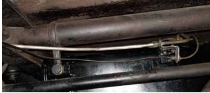
5. Once the pump is mounted, connect it to the fuel tank. I am using 5/16-inch copper/nickel tubing and flare fittings (see "Materials and Supplies" sidebar). No rubber hose. This fuel system should last the life of the car.
