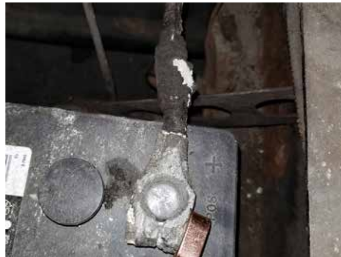
Typical old car battery cable. Time for a replacement.
