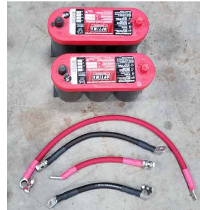
Two Optimas in parallel = 1600 cold cranking amps. This setup will start a diesel bulldozer in Antarctica. Note the large 0-gauge battery cables and built-in battery tender pigtail, which I rounted somewhere discreet but easy to reach.
