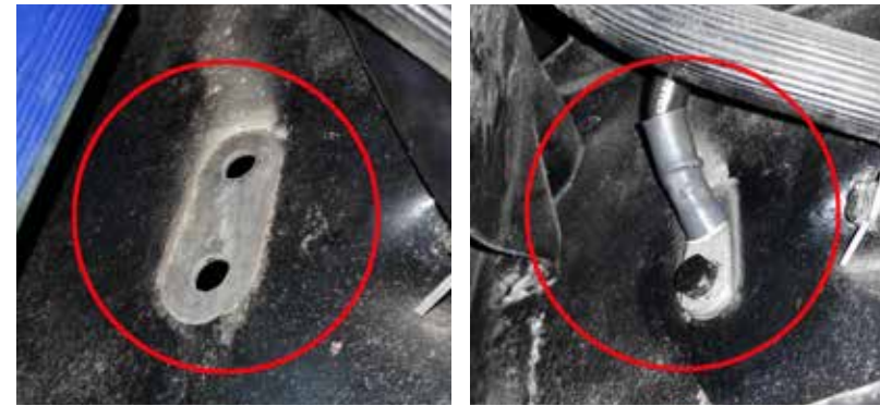
All ground points must be bright, clean metal before installing your new battery cables.
