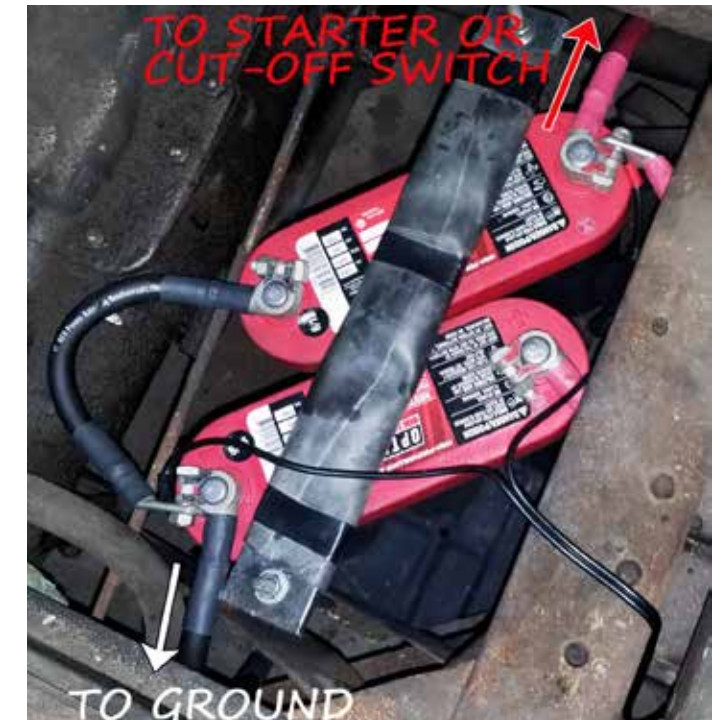
Two Optimas in parallel = 1600 cold cranking amps. This setup will start a diesel bulldozer in Antarctica. Note the large 0-gauge battery cables and built-in battery tender pigtail, which I rounted somewhere discreet but easy to reach.
