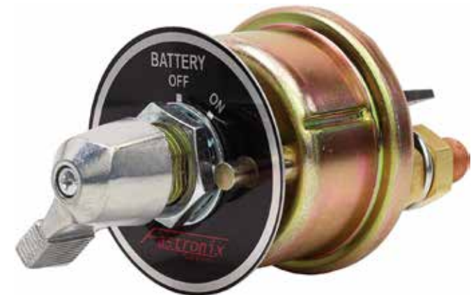
This is the switch you want. It'll handle 300 amps continuously and a whopping 2000 amps for 30 seconds. Costs $50 and weighs a pound.
