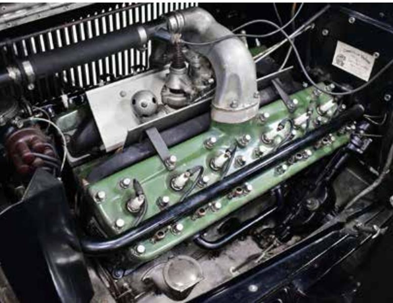
Magnificent 424 cubic inch "Twin Six" engine was far ahead of its time (note the heat shields and spacers added by the owner to fight vapor lock)
