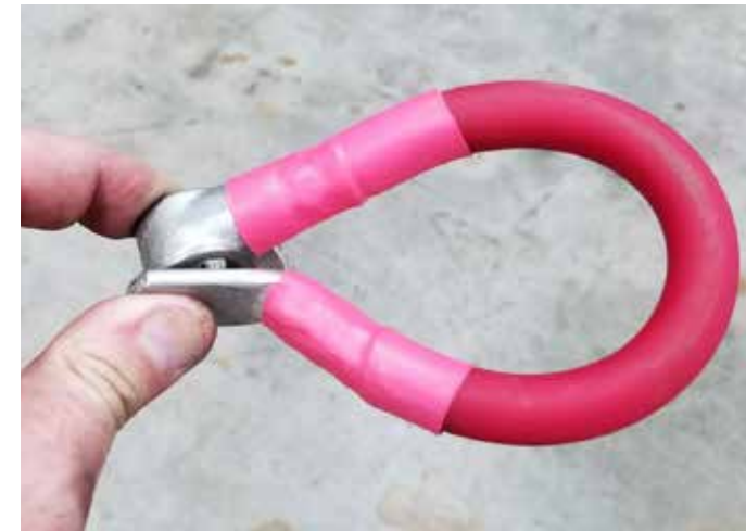
Heavy-gauge battery cables are a MUST on 6-volt electrical systems (check out the awesome flexibility on these cables made by Certified Auto Electric)
