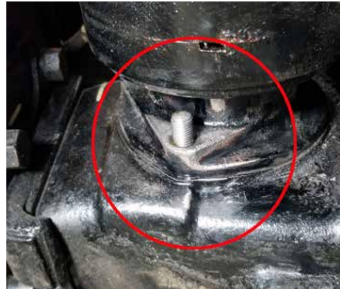
Clean your starter mounting points carefully—this is your ground path. Note the rubber engine mount to the left of the starter.
