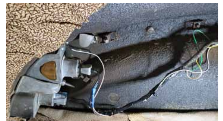
Connect the wires to your existing brake light wiring as shown in the wiring diagram. There are two pairs of wires (power and ground for each half of the Brakelighter). We opted not to use the plastic wire taps included with the kit and instead soldered the wires into the harness near the taillight. For the ground, we used the taillight housing itself, which is also the ground for the factory brake light and turn signal.
