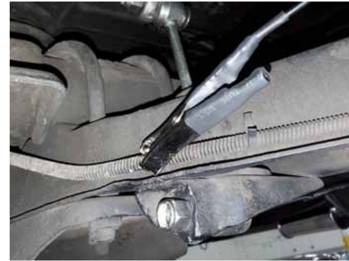
Chassis Ear microphone attached to the Buick's E-brake cable to trace an odd buzzing rattle
