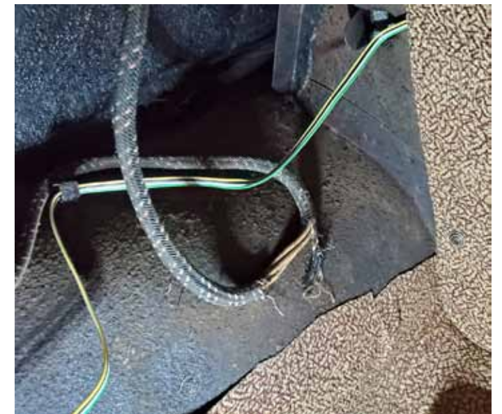
Route the wires (G, B, W, Y) inconspicuously to a place where they can be connected to the taillight wiring. We connected the Buick's wiring in the trunk.
