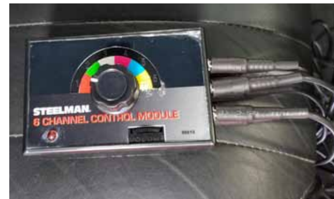
Connect the leads to the control head and locate it in a place where you can change channels as you drive (or have a helper do it)
