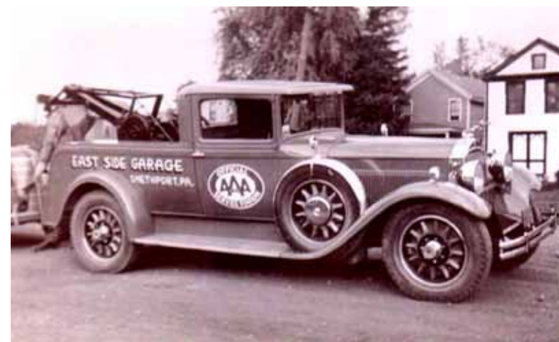
Beautifully built 1930 Packard service car (note how the belt molding continues into the bed).
