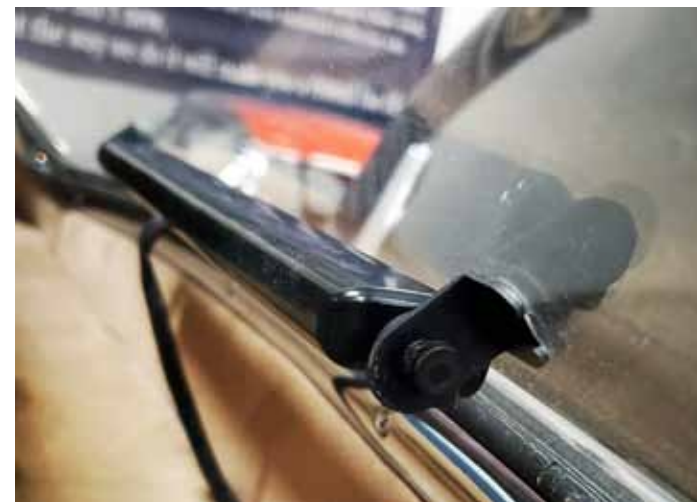
Install the Brakelighter LED housing where it will be most visible. For our Buick with a sloping rear window, we ordered the optional angle brackets.
