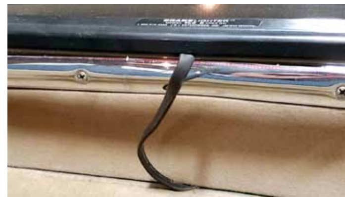
Install the Brakelighter LED housing where it will be most visible. For our Buick with a sloping rear window, we ordered the optional angle brackets.
