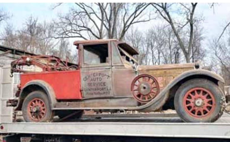
1929 Packard 640 tow truck built from a Holbrook limousine (I've tried twice unsuccessfully to buy this truck—ed.).
