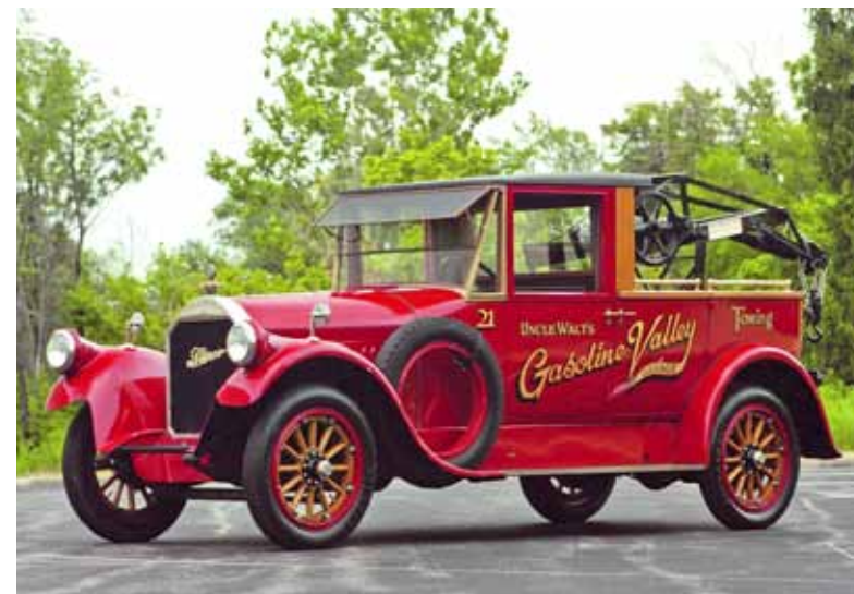
1920s Pierce-Arrow wrecker obviously built from a 4-door sedan (note rear doors still in place and apparently operational).
