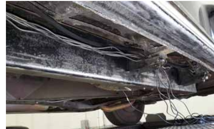
Route the leads to the control head taking care to avoid hot or moving parts. It's only temporary so they don't have to be anchored.
