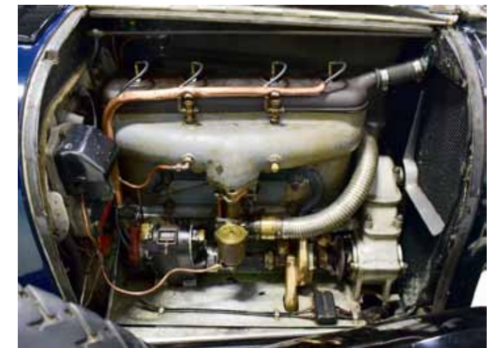
276.5 cubic inch sleeve valve engine has never been apart and runs superbly
