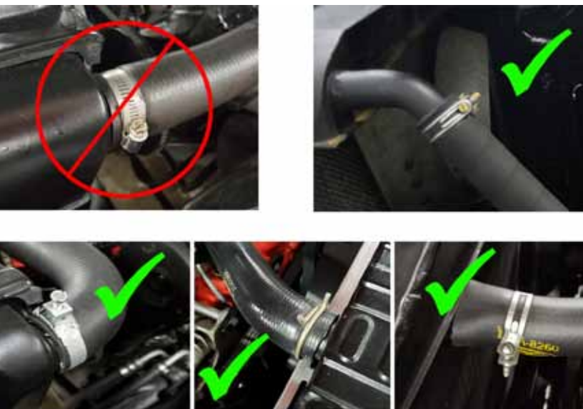
One of the slides dealing with correct vs. incorrect hose clamps on vintage cars.
