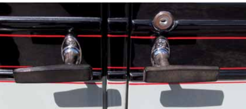
Exterior door handles are made of hard rubber, not metal. Good luck trying to find a set of those today!
