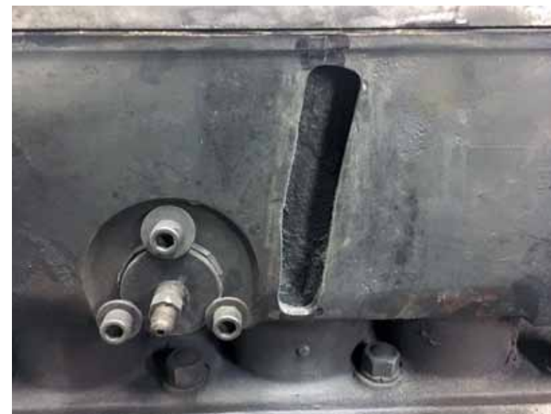
...which required this much material be removed for repair.
