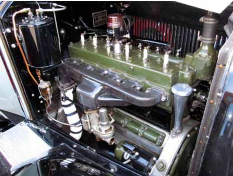
Packard's 241 cubic inch inline-6 was as smooth and torquey as many contemporary V8s.
