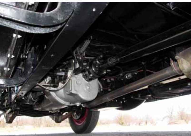
Gracie was as highly detailed underneath as on top. Note that Harry had the entire exhaust system nickel plated to correctly emulate the color of the original steel but to prevent rust from forming in the usual places.
