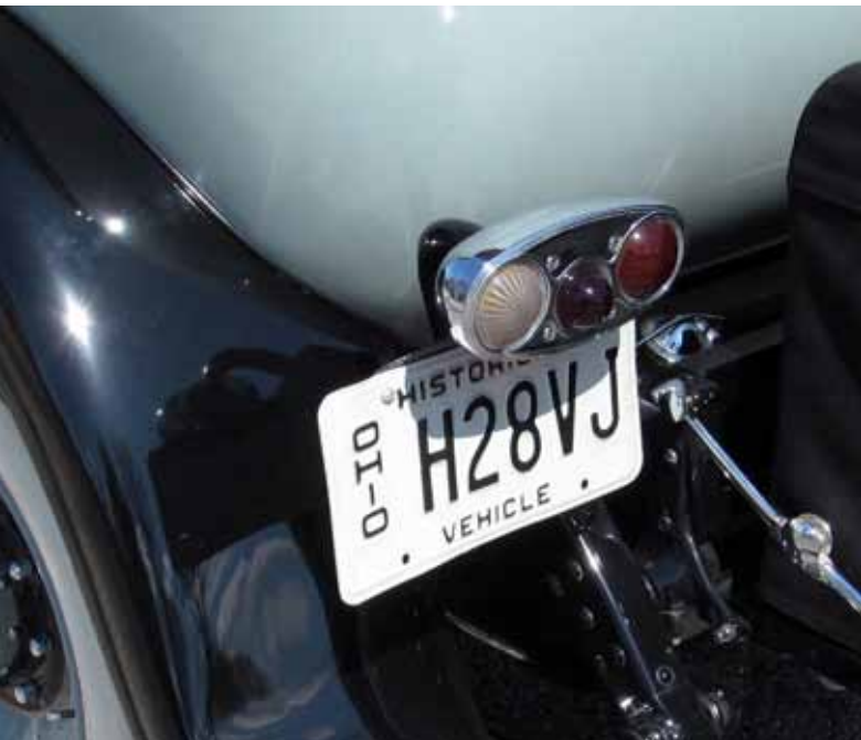
Packard's familiar three-element taillight, which incorporates stop, tail, and back-up light functions.
