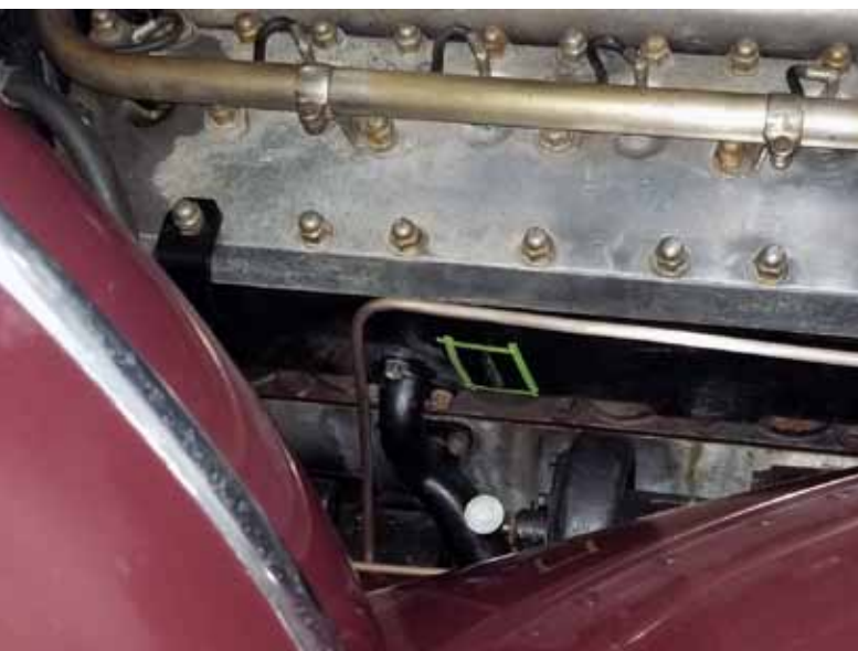
Just a little leak in the side of the block...
