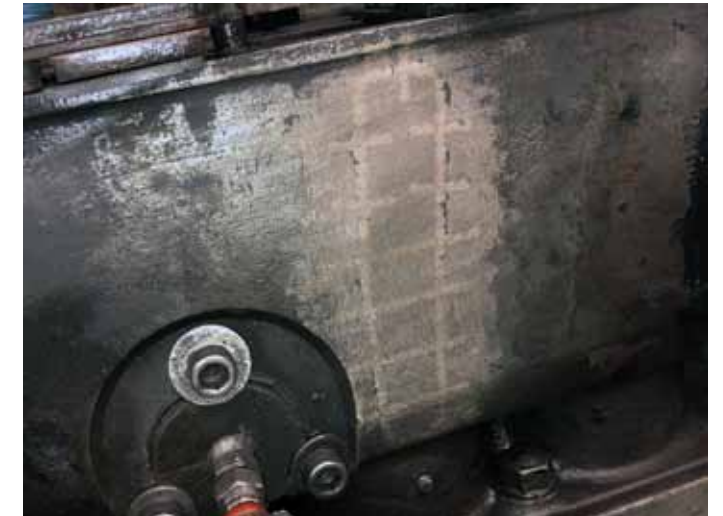
New cast iron "patch" stitched into the side of the Lincoln's block, then ground to match the surface. Note the use of perpendicular locks to hold the patch in place and laces to permanently fill the perimeter.
