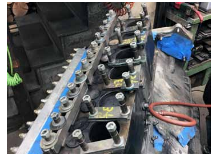
Right cylinder bank being pressure tested. It held 45 PSI for three days. Repair is good.
