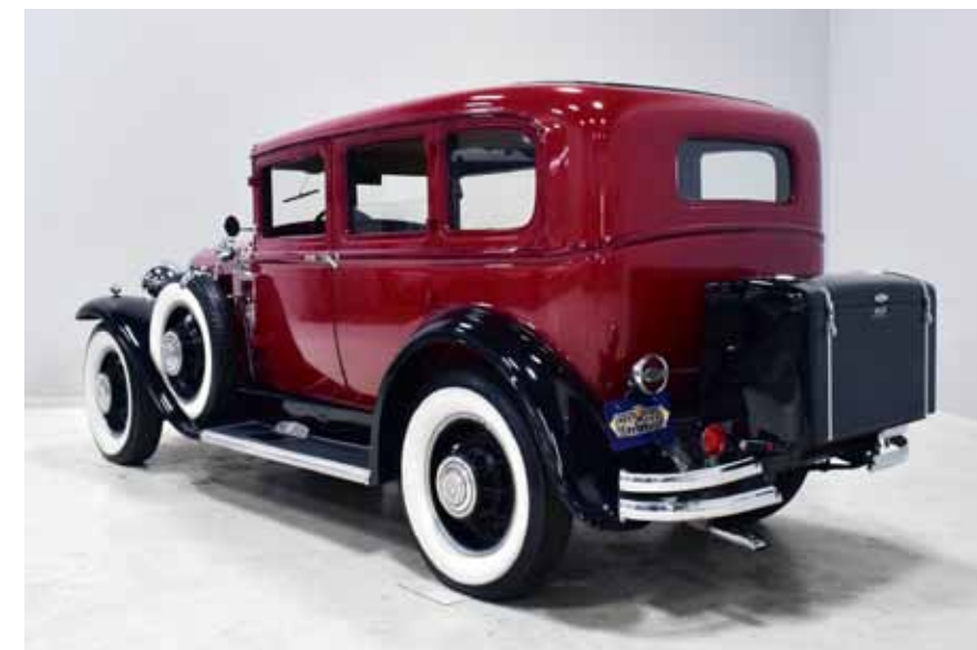
Rear view shows optional trunk rack and trunk. Auxiliary lights and exhaust tip are modern accessories.
