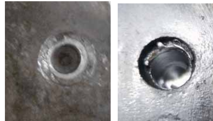
Drill progressively larger holes until there's only a thin shell of the broken stud left.
