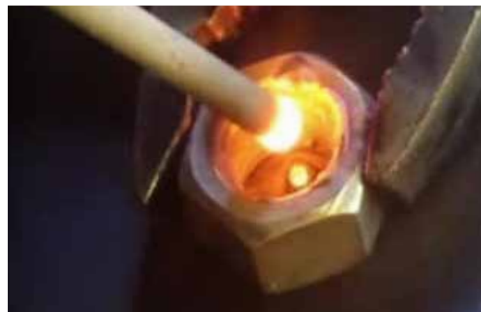
Weld a nut to the broken end...
