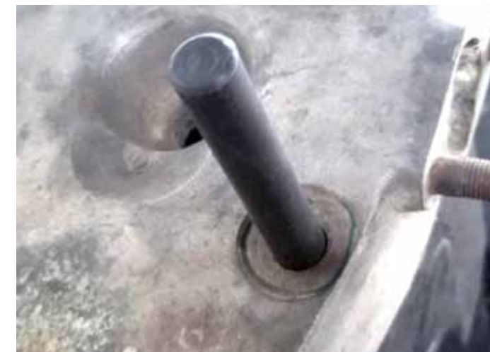
Use a transfer punch and the cylinder head as a guide to hit the center of the broken stud
