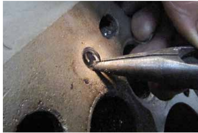
Use a small drift and hammer to knock the last bits of stud out of the threads, then remove the remains with needle-nose pliers
