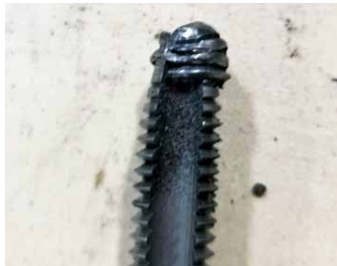
Thread chaser should remove any remaining bits of the stud
