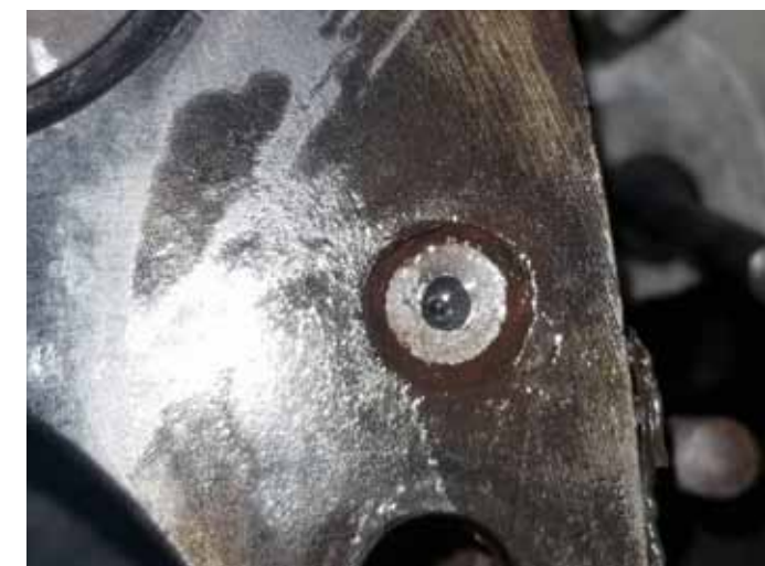
Transfer punch makes a neat pilot hole in the center
