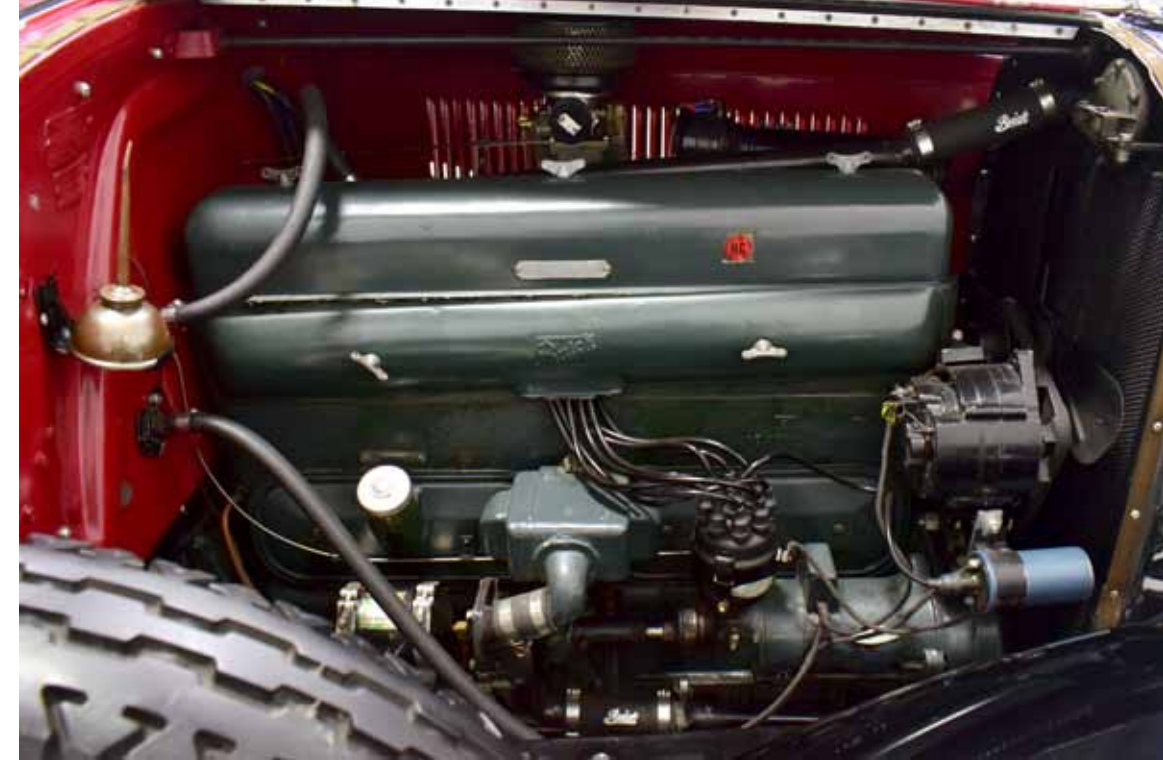
344 cubic inch OHV straight-8 is well-engineered, durable, and powerful. Note non-stock alternator and downdraft carburetor.
