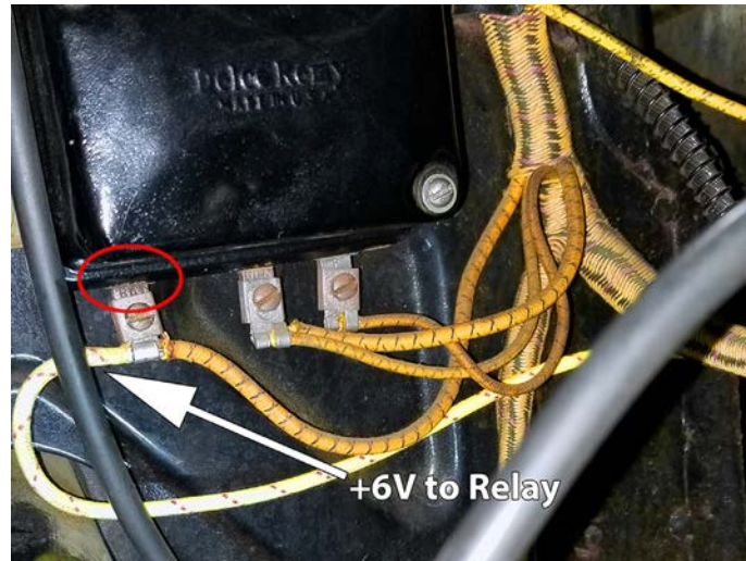
The BAT terminal on the voltage regulator provides a full 6 volts to the relay
