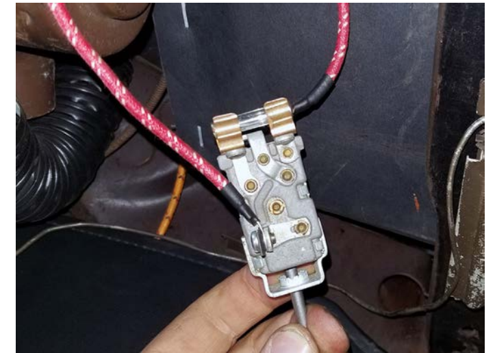
NOS factory fog light switch before installation in the dash
