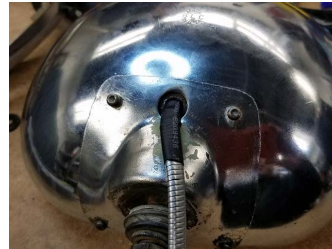
12/2 armored cable with some shrink-wrap as a strain relief looks quite correct and should last many years
