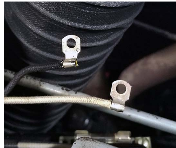
Flag terminals are period-correct and handy, but soldering is required
