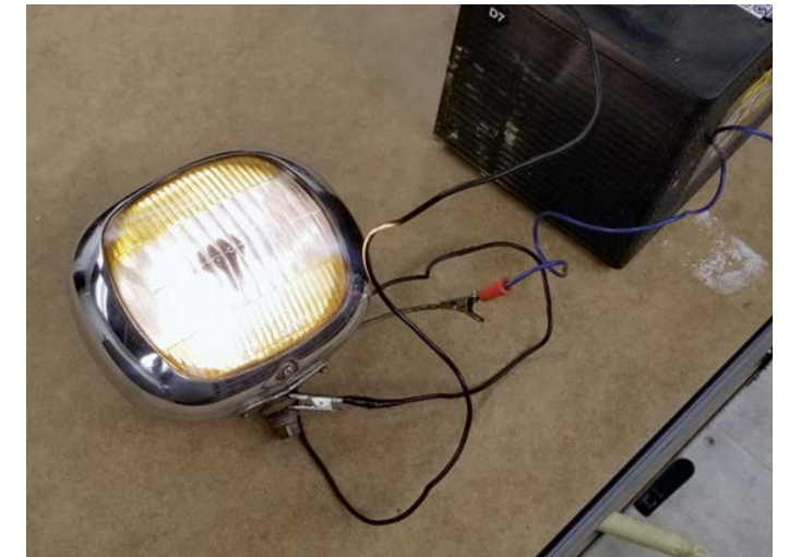
Bench testing the rebuilt fog lights
