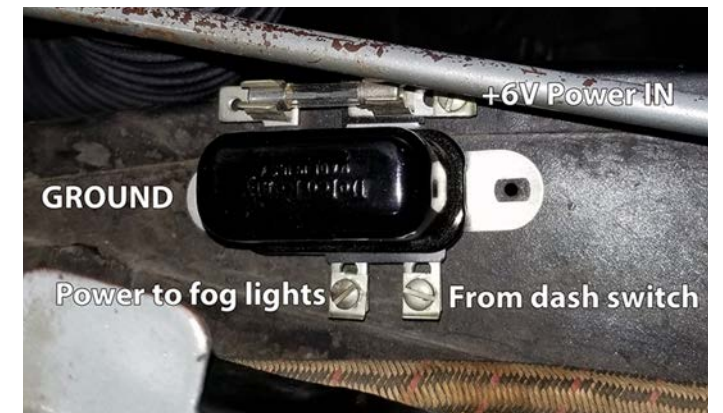
Relay mounting location and connections
