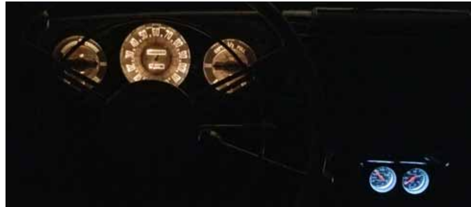
Soft, yellow glow of incandescents in original gauges bright blue-white glow of modern gauges with LEDs
