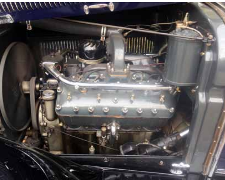
Lincoln's durable 384 cubic inch "fork and blade" V8
