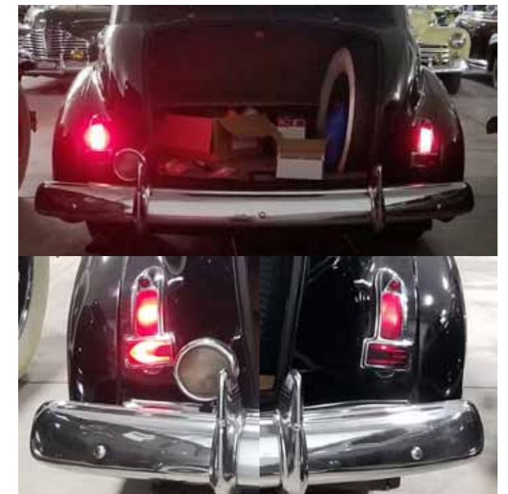
Brake and turn signals show significant improvement
