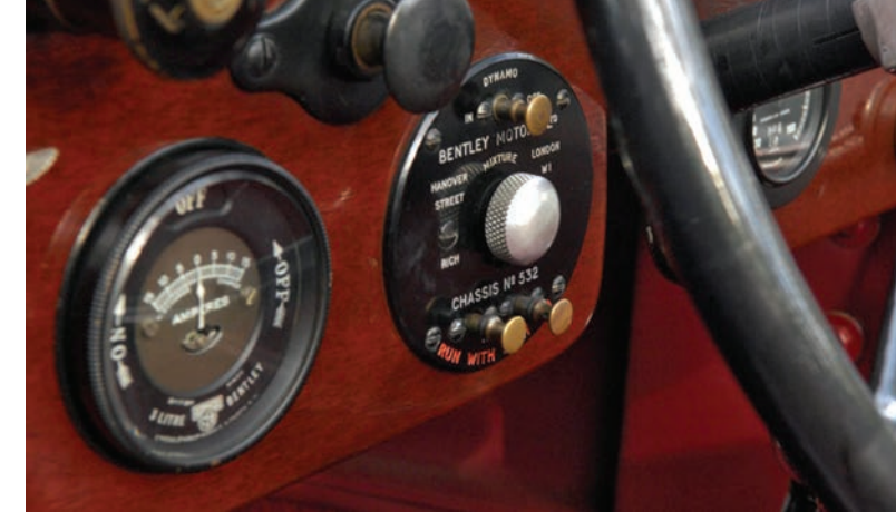
Main ignition switch surrounds ammeter. Dual ignition system buttons below mixture knob, and even the generator is switchable for maximum performance
