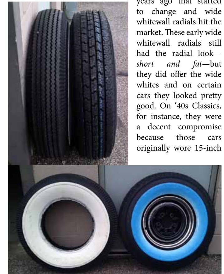
7.50-16 bias-ply (left) and 750R16 radial. Note that the radial is very close in overall height and width.
