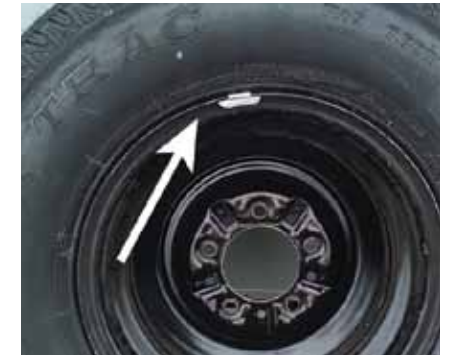
Radials typically balance easily, with my 1941 Buick's wheels needing only one small weight.
