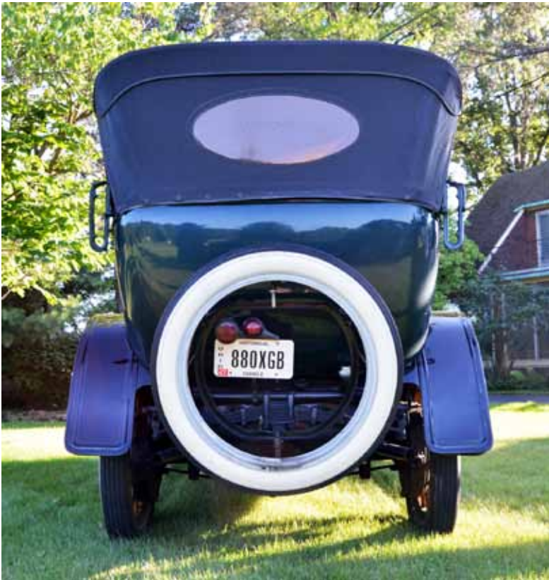
Rear-mounted spare tire was optional Additional taillight added for safety
