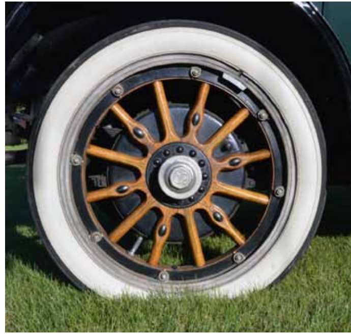
Wood spoke wheel with integral brake drum
