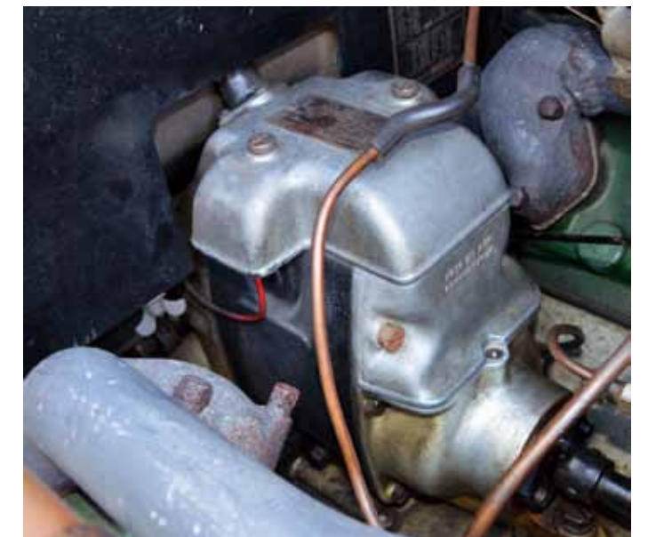
Heart of the electrical system: the Delco self-starter/generator at the rear of the engine
