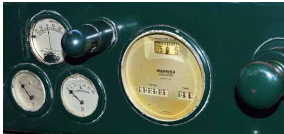
Instrumentation with manual fuel pump knob on right
