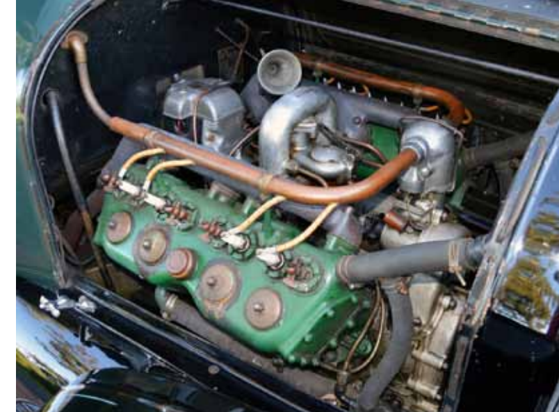
314 cubic inch V8 makes 77 horsepower
