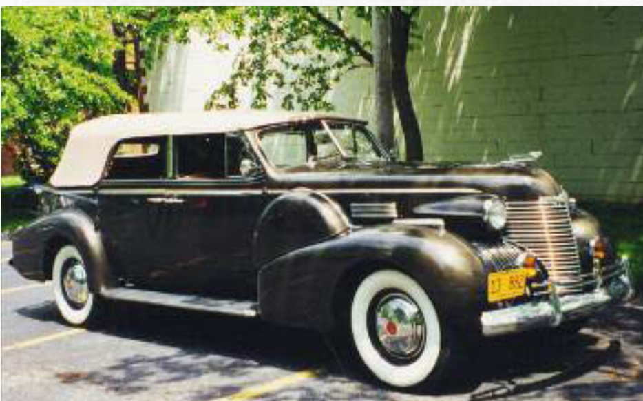
1940 Cadillac V-8 convertible sedan. Same body and chassis as the 1938-40 V-16 cars. The main styling difference is the grill.
