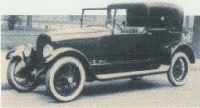
Holbrook Co. of Hudson, New York, built this stylish town car on a Marmon 34 chassis.
