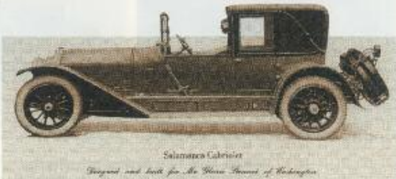
Locomobile model 48, circa 1917, with coachwork by deCausse. The narrow cowl section saw the emergency brake handle mounted outside the body.
