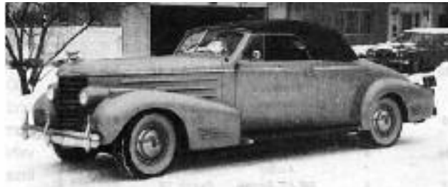
This 1938 Cadillac Series 90 convertible coupe was fitted with power steering and an automatic transmission behind its original flathead V-16 engine by the GM Tech Center for the car's original owner.
